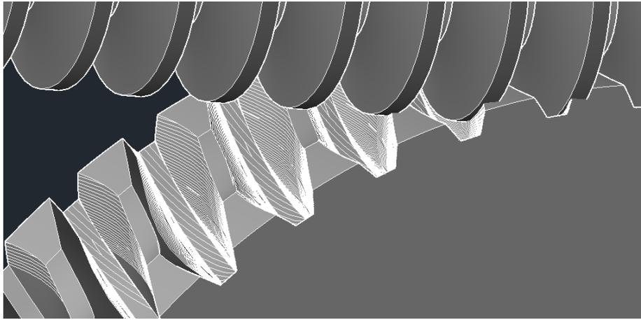
Figure 5: Shaping of worm wheel tool flank
